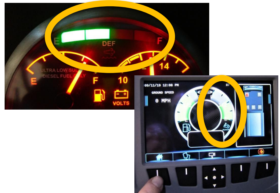
DEF level display located above fuel gauge on dash, as a separate gauge, or within a vehicle system screen.
