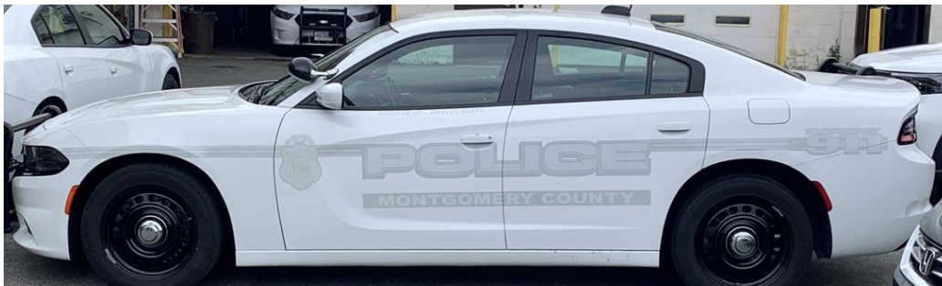
Figure 40 - Police car with “ghost graphics” that are faint during the day but highly reflective at night.
