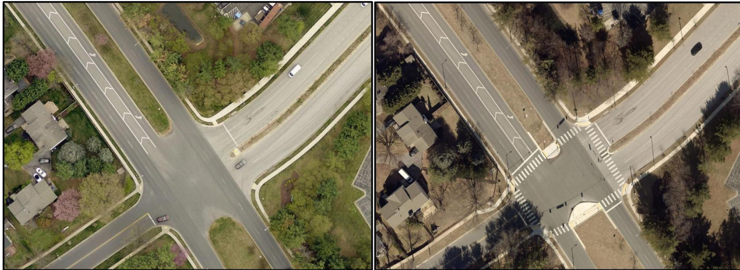
Figure 13 - Before and after at the intersection of Crystal Rock Drive at Waters Landing Drive. Along with a new traffic signal, new high visibility crosswalks and raised concrete medians along Crystal Rock Drive were installed.
