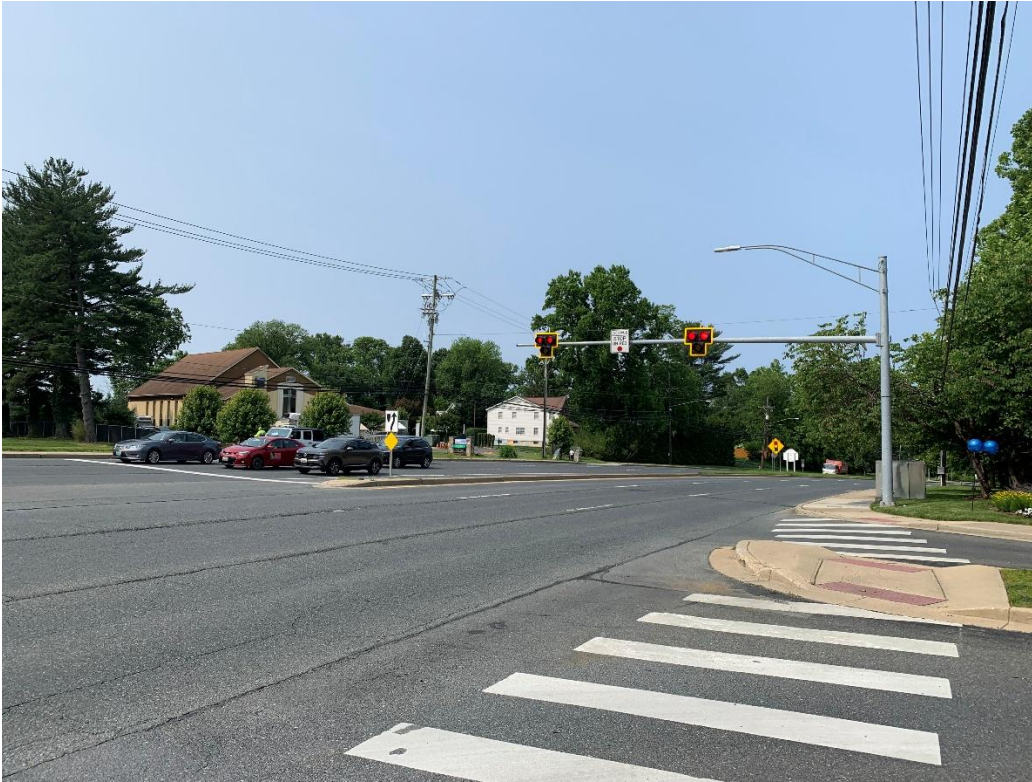
Figure 22 - Signals and beacons with retroreflective borders improve conspicuity at night.
